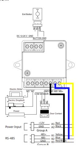
After connecting the LTH-SM1 to the terminal, login to the terminal and access the configuration settings. In the settings, navigate to Access Control -> RS-485. Change the Peripheral type to Extension Module and save. The default RS-485 settings are correct for the LTH-SM1. The device will reboot and the LTH-SM1 will be able to unlock the door.
