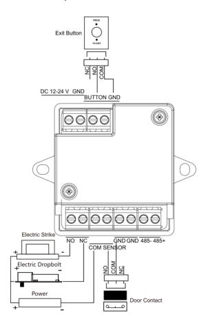
To connect the LTH-SM1 with either the LTK3411FM or the LTH401M-WIFI, the RS-485 terminals must be wired to the corresponding RS-485 wires on the terminals' wire harness. This is shown below.
